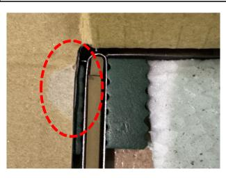
BASED ON DIE-BLADE CHECKING THE PORTION OF FEEL OFF AND DIE-BLADE AS A WHOLE ARE STILL IN A GOOD CONDITION
